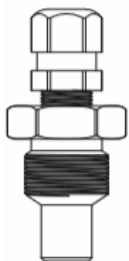
Gas Valve, 3,000 PSI
